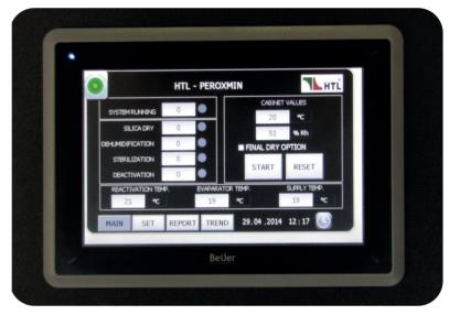
All operation parameters of the cycle can thus easily be set and are protocolled by a GMP compliant printer output function.
